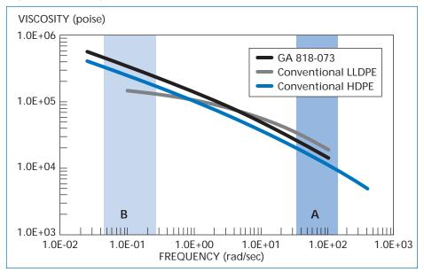
All polyethylene resins display a phenomenon known as shear thinning. As a resin is pushed faster through an extruder at high shear rates (high frequency), it appears to have a decreasing viscosity. The amount of "shear thinning" that occurs is largely controlled by the breadth of the resin's molecular weight distribution. Broad molecular weight distribution resins display greater shear thinning, which translates into easier extrusion.
