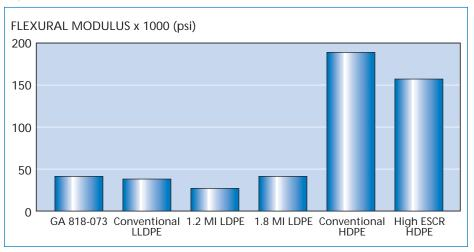
Figure 1. Comparative flexural modulus data (ASTM D-790)
