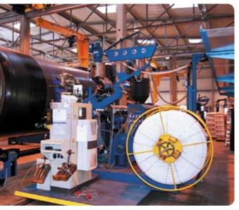
Fig. 3: Production of spirally wound pipes at FRANK & Krah GmbH as per PAS 1065 / DIN 16961
