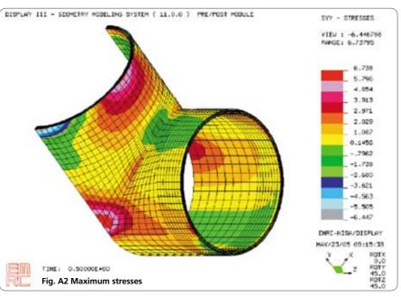
Fig. 7: Finite element model, tee DN 1400, LGA Nuremberg <sup>6</sup>
