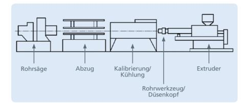
Fig. 2: Production process for extruded pipes as per DIN 8074
