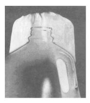
Figure 4: With the flash ending far too high on the handle, a blowout and a useless bottle result.
