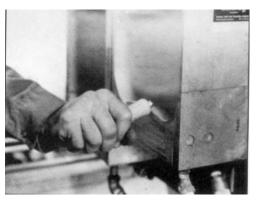
Figure 2: Apply the tool with both force and judgment to sharpen worn pinch-offs.
